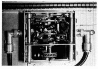
Input network is built as a separate module.
